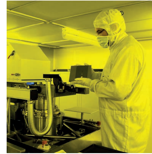
HEIDENHAIN glass scales, which feature accuracies in the micrometer range, are manufactured in the Mastering department. Our precise manufacturing processes place highly stringent demands on the quality and reliability of our clean-room technology.
